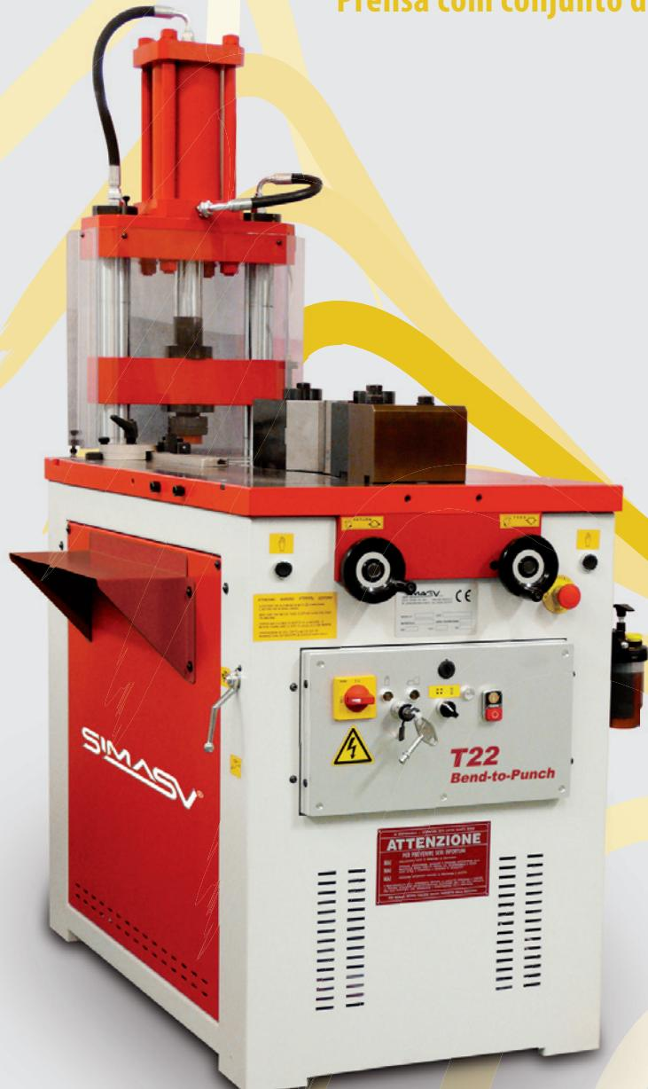
Bending press with punching unit
