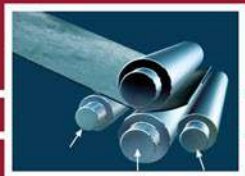
2. Raise the front side roll. Prebend and roll.
