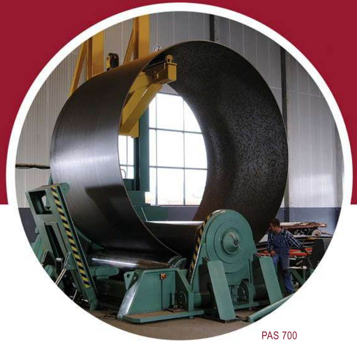
PAS 700 producing wind mill towers
