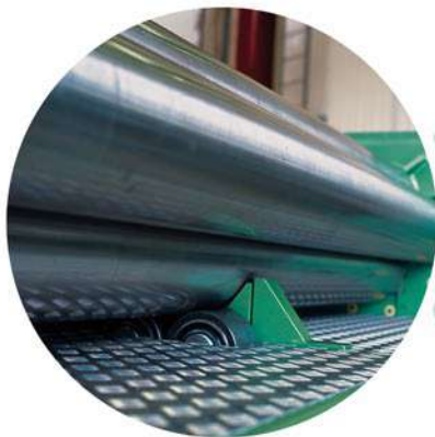
Adjustable support rolls for the lower roll
