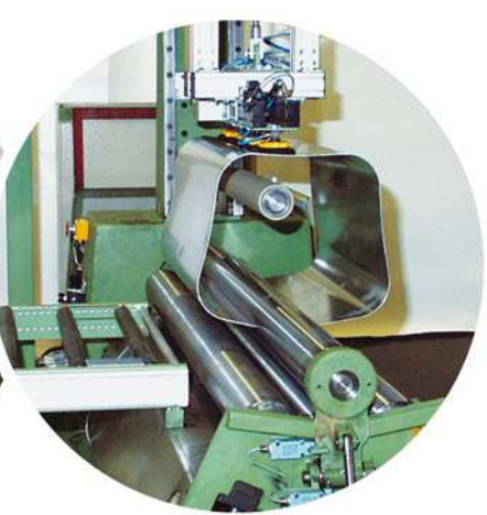
Automatic outfeeding of finished tank body
