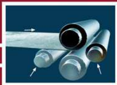
3. Lower the front side roll and raise the rear side roll until it reaches the prebent edge.
