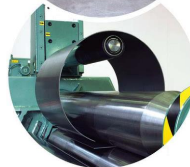
PAS with lifting roll to avoid double plate
