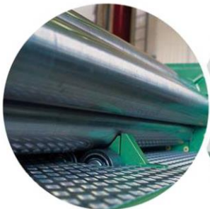
Adjustable support rolls for the lower roll
