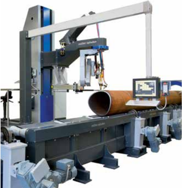
Motorized roller conveyor for pipes with a maximum diameter of 1,524 mm and a maximum weight of 15 tonnes
