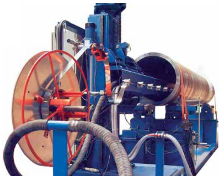
Internal welding jig for the submerged arc welding of longitudinal seams in pipes
