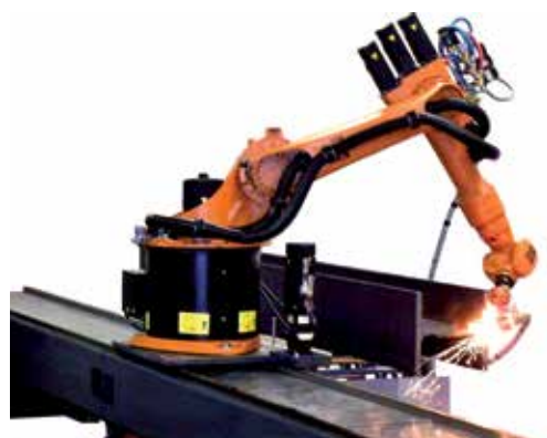
Pipe profile cutting machine RB 950/2500/6 Heavy-Duty with 6 CNC axes for round pipes with a maximum diameter of 2,540 mm
