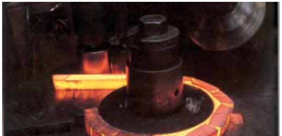
Rotating Table Ring Rolling Machines, ideal for flat and angle bars used as flanges and bearing housings. Capacities up to 70.000 square mm cross-section.
