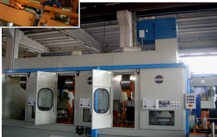
Below: machine provided with cabin and air-liquid exhauster placed on the top of the cabin
