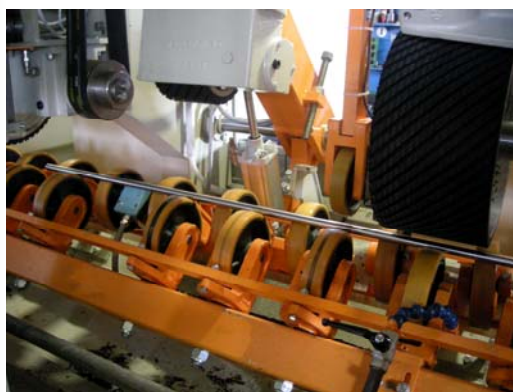
On the right: detail of the roller conveyor along the machine
