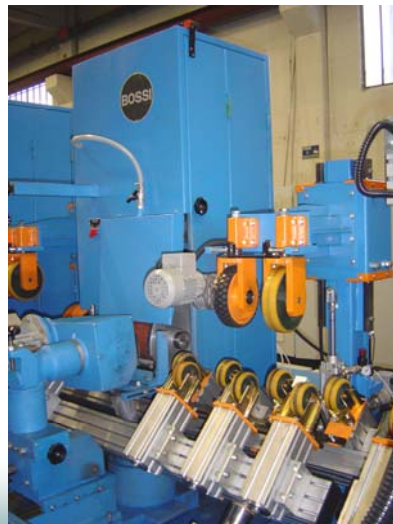
Detail of the grinding unit working with abrasive belt
