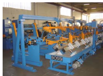
Automatic bundle loader and roller conveyor Mod. H made of aluminium for pieces with lengths from 3 up to 8 meters
