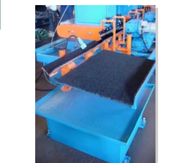
Unloading table covered with bristles against scratches
