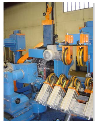
Detail of mop unit, aluminium roller conveyor along the machine and pinch-roll with double wheel
