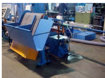
Revolver loader for pieces with small diameters
