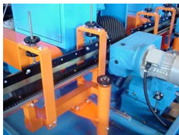
V-guides, covered with bristles against scratches, with upper holding blades
