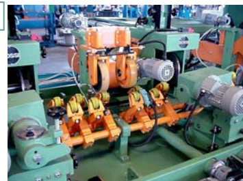
Compass roller conveyors Mod. L, with rolls Ø 70 mm. and motorised pressing roll with double wheel
